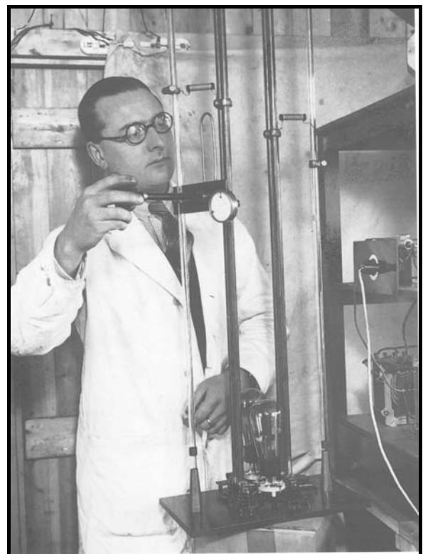
George Brown G5BJ works on a VHF Lecher Line transmitter (G6SL) in the roof-top laboratory at Stratton's Balmoral Works, 1935. Signals were received in New York.
